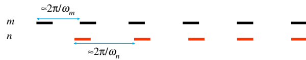
Figure 2. Schematic timelines show signals of two oscillators, each referenced to absolute time, as generated by a phase-oscillator model with the interaction function \Gamma_{nm}(\theta_m - \theta_n) = K \cdot \sin(\theta_m - \theta_n) . If m and n have similar natural frequencies, i.e. (\omega_m - \omega_n) is sufficiently smaller than the coupling strength K , synchrony is attained after multiple cycles.
